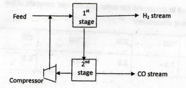
The system is designed to recover 93.2 % CO with 98 mole% purity. Recycle stream is kept at 3000 mol/h for a fresh feed rate of 5000 mol/h. This requirement is stipulated to achieve 1:1 mole ratio of H<sub>2</sub>/CO in the feed to second stage. Find
